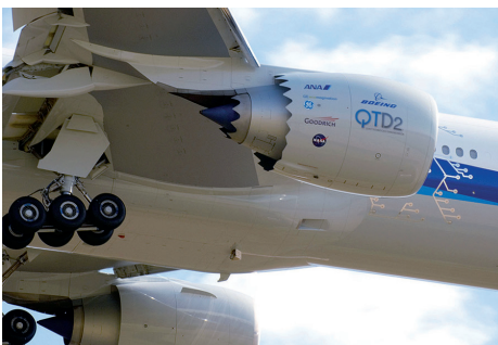
Testing on this All Nippon Airways 777-300ER showed that the chevron shape of the engine nozzle helps reduce noise. © Boeing. All Rights Reserved.
